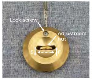
After a week (or a month in case your clock is fitted with a 30-days movement) read the time shown by the clock as well as the correct time. This will show whether the clock goes at the correct speed or whether it gains or lags.
